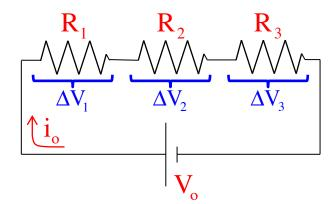
The idea behind  $R_{equ}$  is to find the single resistor that can take the place of all the resistors in the system. In other words, the single resistor that, when put across  $V_o$  will draw  $i_o$
