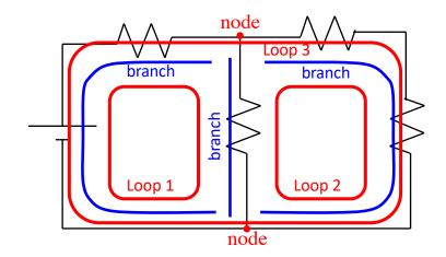
A node: A junction where current can split up or be added to.
