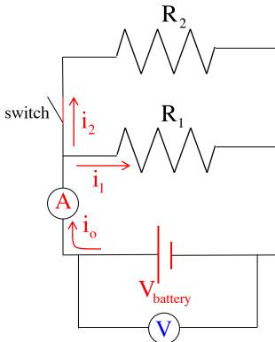
c.) Here's the rub: if you carry this experiment out in the real world, the light bulb associated with  $R_1$  will actually dim suggesting that the current through  $R_1$  has diminished. So what's going on?
