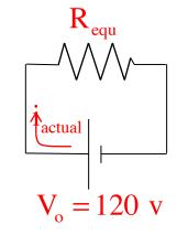
which is way too little current to power the 100 W bulb and just barely enough to power the 40 W bulb!
