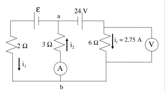
b.) What is the voltage difference between *Points a* and b?
